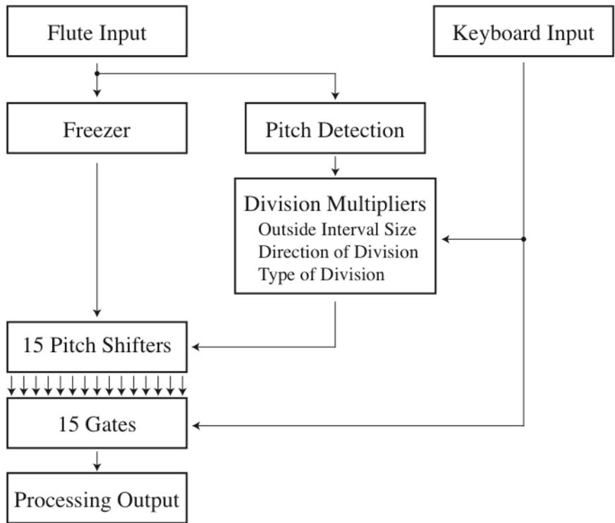
FIGURE 17. A block diagram of the computer processing used in *Anomaly*.
